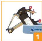
Tip-up tape head simplifies roll replacement
