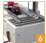
Horizontal self-centering in-feed guides
